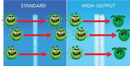
Standard Low-Output UVC lamps can only kill germs on surfaces inside your HVAC system, while High-Output UVC lamps on kill on these surfaces as well as sterlize aireborne viruses, bacteria and germs as they pass by the lamp, rendering them harmless and incapable of reproducing.
